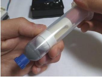
Push the piston inside while squeezing the sides of the barrel with the other hand. Trapped air will escape through the small gap between the syringe walls and the piston, you can feel when this is happening.
