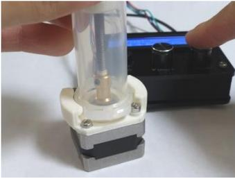
Line up the fins of the syringe and press down the right knob to lower it into position.
