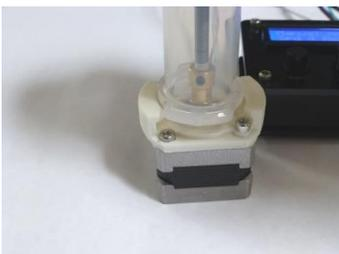
Then thread the barrel in the shaft of the motor as far down as you can.
