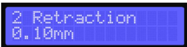
This is the distance the piston will retract automatically after dispensing, essential to prevent oozing and dripping. Typical values are between 0.10 and 0.20mm
