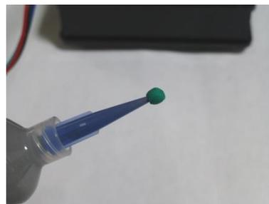
The tips themselves can also be cleaned: remove the paste with a toothpick and then with a rolled up napkin wipe the inside, a couple of drops of isopropyl alcohol help a lot.
