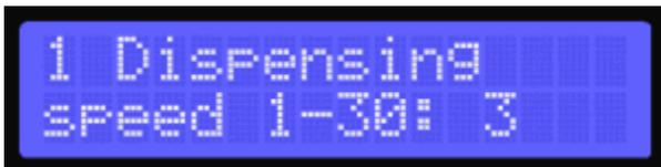
Range from 1 to 30. For high viscosity fluids typical values are between 2 and 5, medium and low viscosity use 5 to 20. Above 20 is recommended for quick movements of the piston.
