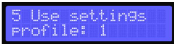
Displays the current active profile. A “profile” is a set of parameters that is saved in the internal memory, since each fluid and tip combination (even pad size) will have different speed and retraction values this is an easy way to change between them. When you change profile its values are immediately loaded.
