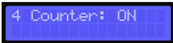
Enables or disables the counter on the main screen, switching on and off also resets the count.
